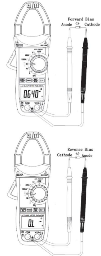
Figure 3-6 Measuring Diode
